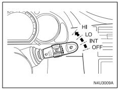
Use the windshield wiper/washer lever to operate the windshield wipers.
